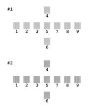
8. Look at the alignment pattern in each set and find the patch which is most evenly printed, with no noticeable streaks or lines.
